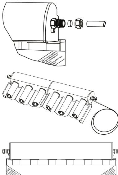
The flow or return pipe can be connected to the collector on the left or on the right, as selected.
