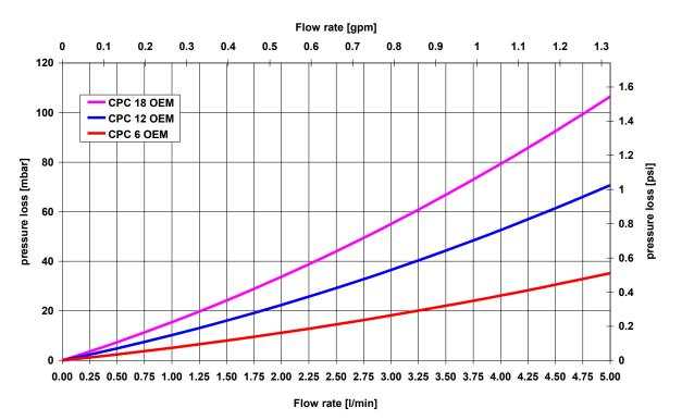
Pressure loss of tube collector CPC 6/12/18 INOX Heat transfer medium: Tyfocor LS; medium temperature: 100°F
