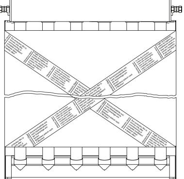
Upon delivery, the collector is covered by a sun protection film. This facilitates trouble-free commissioning of the solar energy system even in strong sunlight. It prevents the heat transfer medium being vaporized, rendering commissioning impossible. Remove the sun protection sheet after commissioning.
