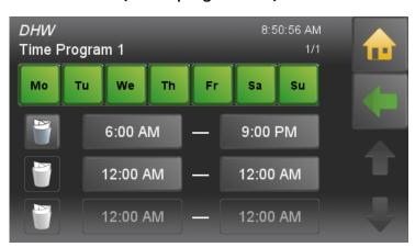
The domestic hot water time programme works the same way like the heating circuit time programme.
