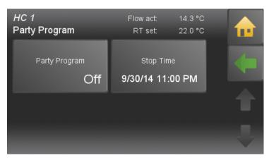
The party function is basically inactive. Enter the time until the room temperature heating should be heated. Activate the Party function. The heating time is extended up to the indicated time. Then the party function deactivates itself automatically.
