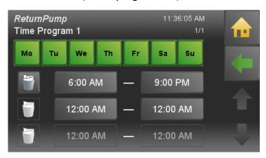
The DHW return pump time programme works the same way like the heating circuit time programme.
