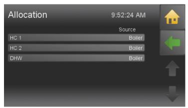
In the menu item **Allocation** you see which heating circuits are allocated to the boiler or to the accumulatores.
