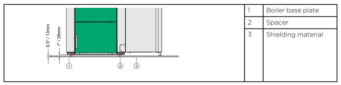
The spacer must be able to support the weight of the boiler and has to be non combustable. The shielding material must be equivalent to a  $\frac{1}{2}$  in / 13mm micro board with a K-value of 0.49 (W/m K) (R-value of 1.02 Km2/W) or greater. For more information contact Maine Energy Systems.
